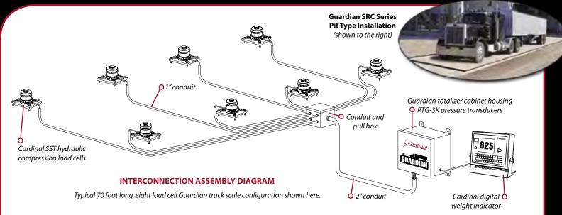
The Guardian all-stainless steel hydraulic compression load cell is the ideal solution to those applications requiring superb accuracy in a hostile environment.
